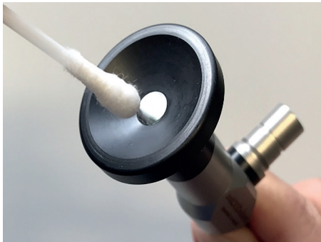
Fig. 4: Cleaning the Proximal Window
