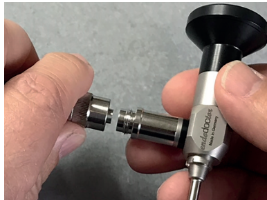
Fig. 5: Connection of an optical fibre cable with thread (compatible to the suppliers *Storz, *Olympus)
