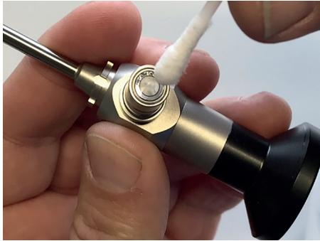
Fig. 3: Cleaning the light guide attachment
