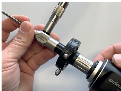
Fig. 9: Placing an endoscopy camera on the standardized eyepiece funnel
