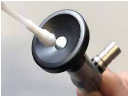
Fig. 4: Cleaning the Proximal Window
