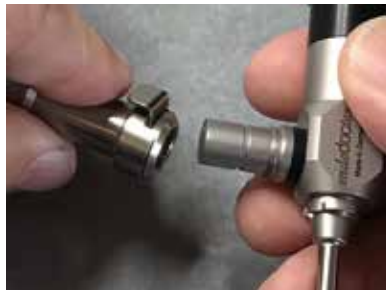
Fig. 6: Connection of a fibre optic cable with snap mechanism (compatible with *Wolf). The first sleeve of the fibre optic cable attachment is removed
